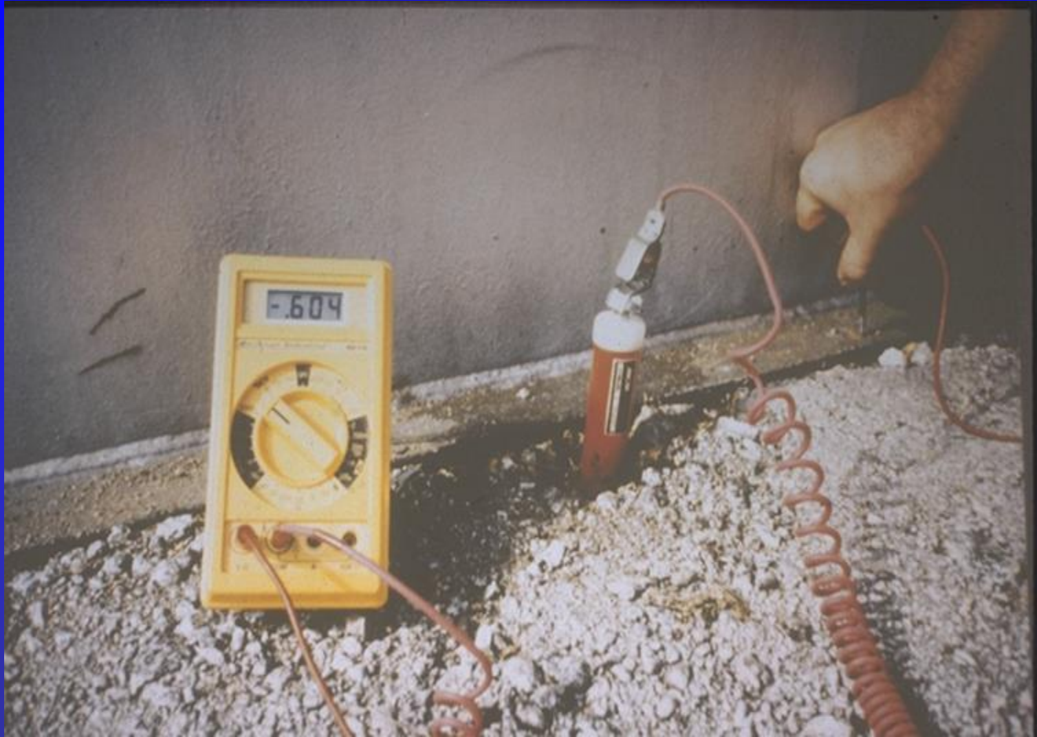
Tank to Soil Potential Measurements
