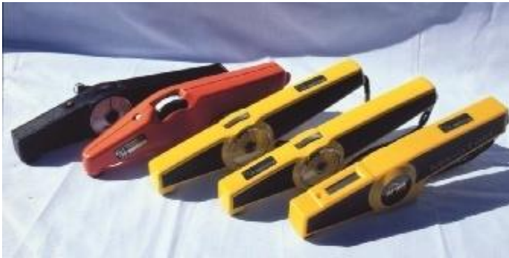
Type 1 – Magnetic Pull-off Gages
