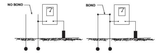
INTERFERING RECTIFIER OFF INTERFERING RECTIFIER ON -METER READING IS IDENTICAL TO THAT AT LEFT
