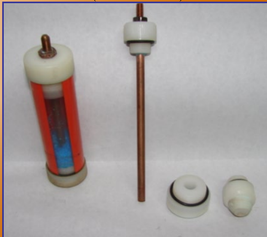
Standard Reference Half Cell (Cu-CuSO 4 Electrode)
