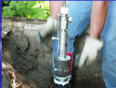
Open top valve, insert the rod to the designated marked location.
